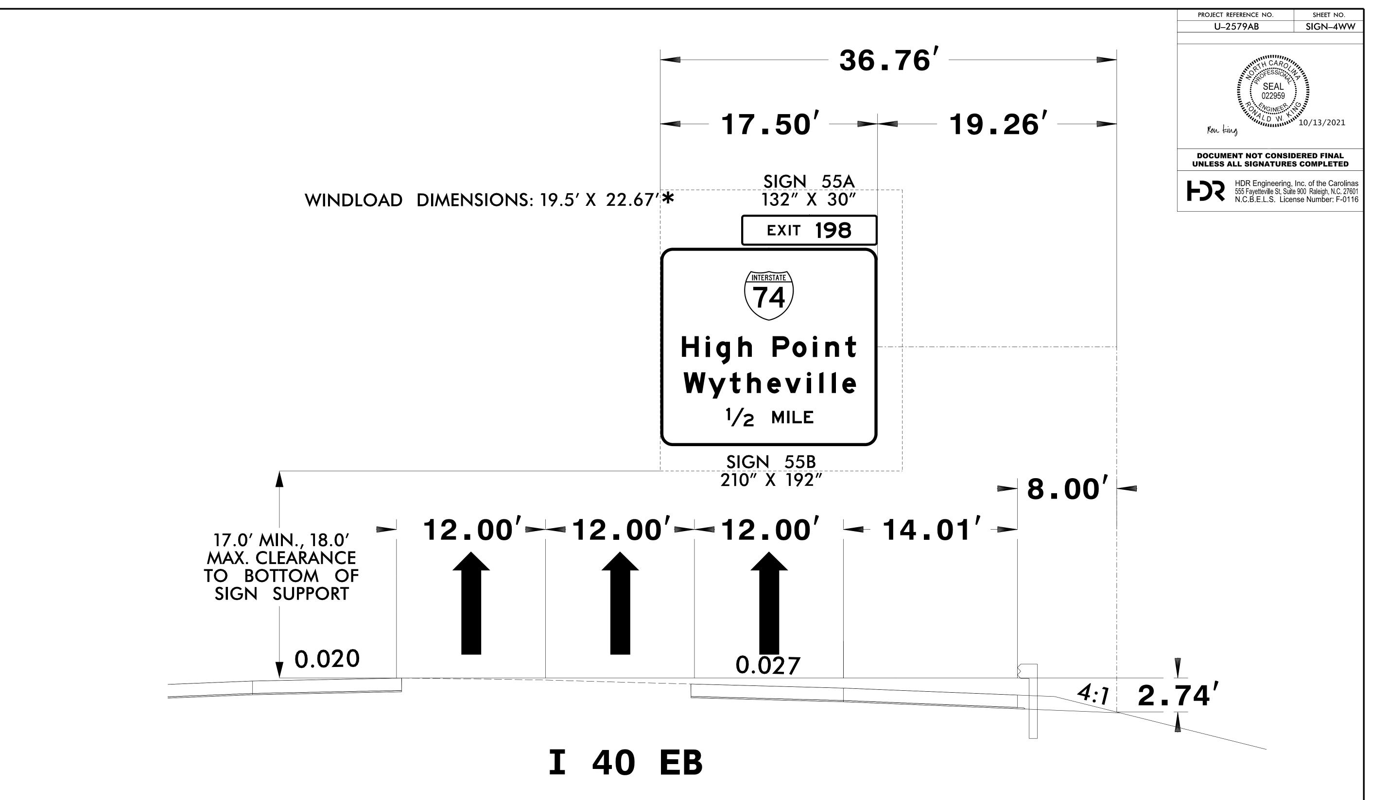
IF THE CONTRACTOR BIDS ALUMINUM SIGN STRUCTURE, EACH SHALL BE PROVIDED WITH AN APPROVED HIGHWAY TRUSS DAMPER DEVICE IN ACCORDANCE WITH AASHTO SPECIFICATIONS.
