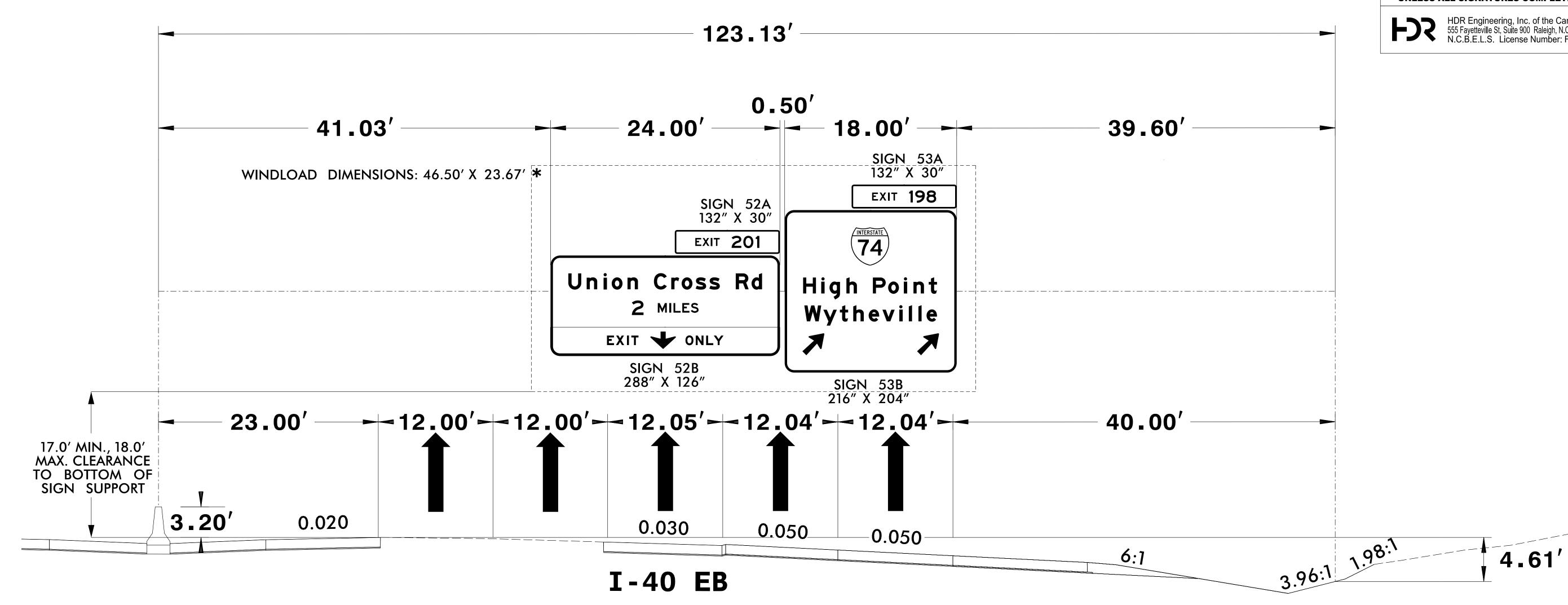
IF THE CONTRACTOR BIDS ALUMINUM SIGN STRUCTURE, EACH SHALL BE PROVIDED WITH AN APPROVED HIGHWAY TRUSS DAMPER DEVICE IN ACCORDANCE WITH AASHTO SPECIFICATIONS.
