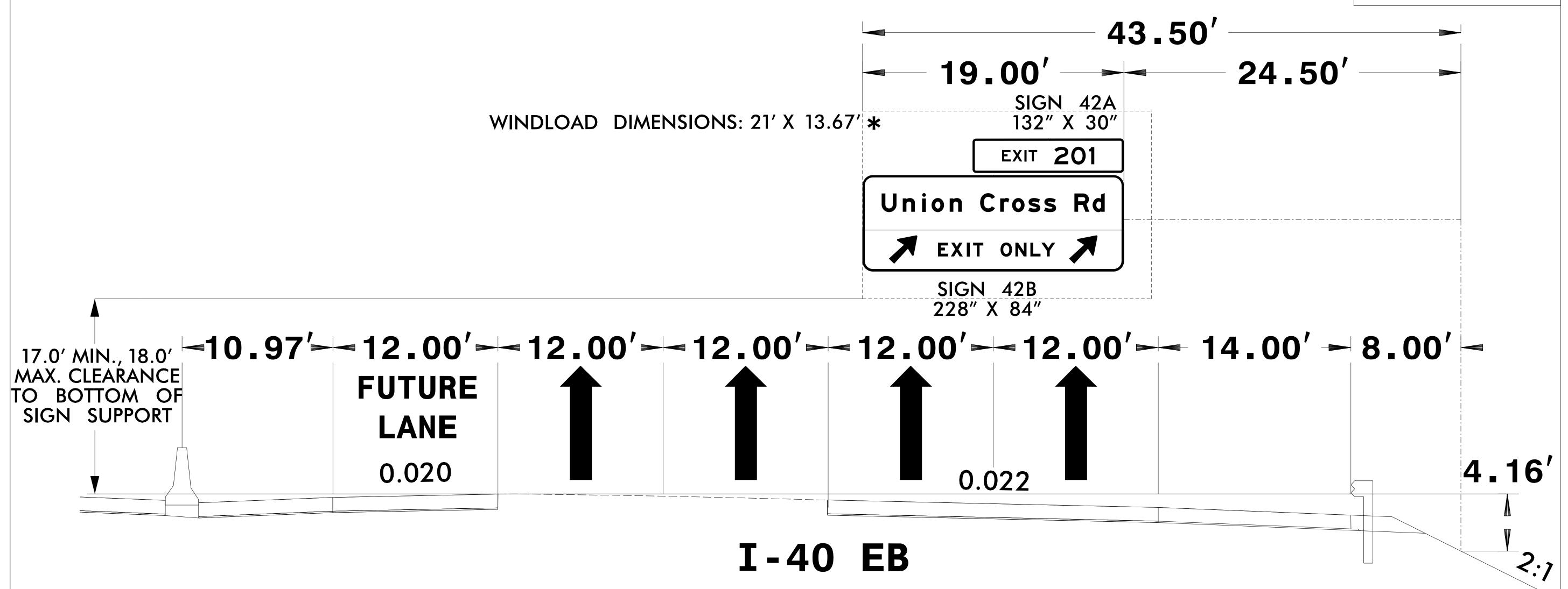
IF THE CONTRACTOR BIDS ALUMINUM SIGN STRUCTURE, EACH SHALL BE PROVIDED WITH AN APPROVED HIGHWAY TRUSS DAMPER DEVICE IN ACCORDANCE WITH AASHTO SPECIFICATIONS.
