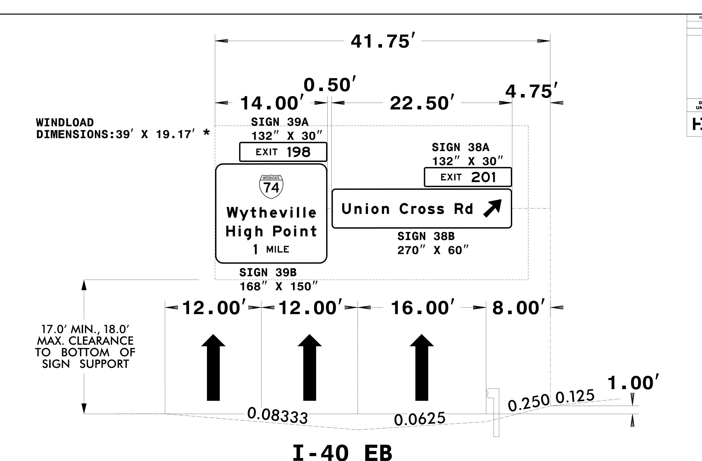
IF THE CONTRACTOR BIDS ALUMINUM SIGN STRUCTURE, EACH SHALL BE PROVIDED WITH AN APPROVED HIGHWAY TRUSS DAMPER DEVICE IN ACCORDANCE WITH AASHTO SPECIFICATIONS.
