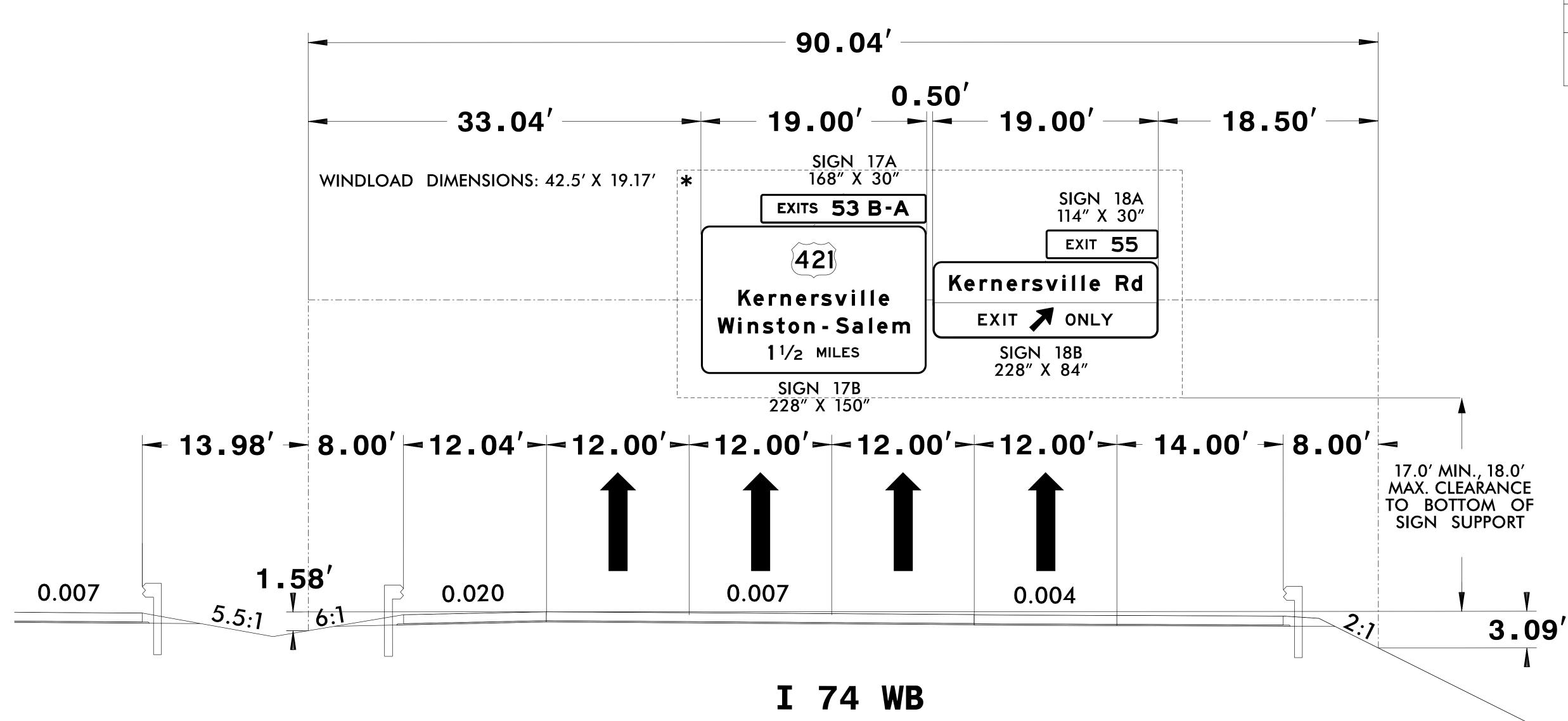
IF THE CONTRACTOR BIDS ALUMINUM SIGN STRUCTURE, EACH SHALL BE PROVIDED WITH AN APPROVED HIGHWAY TRUSS DAMPER DEVICE IN ACCORDANCE WITH AASHTO SPECIFICATIONS.
