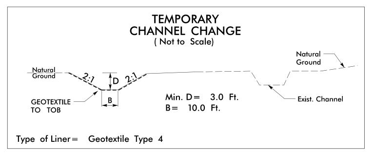
NOTE: CONTRACTOR TO USE BERMS AS NEEDED TO MAINTAIN A MINIMUM 3' DEPTH OF THE TEMPORARY CHANNEL CHANGE.
