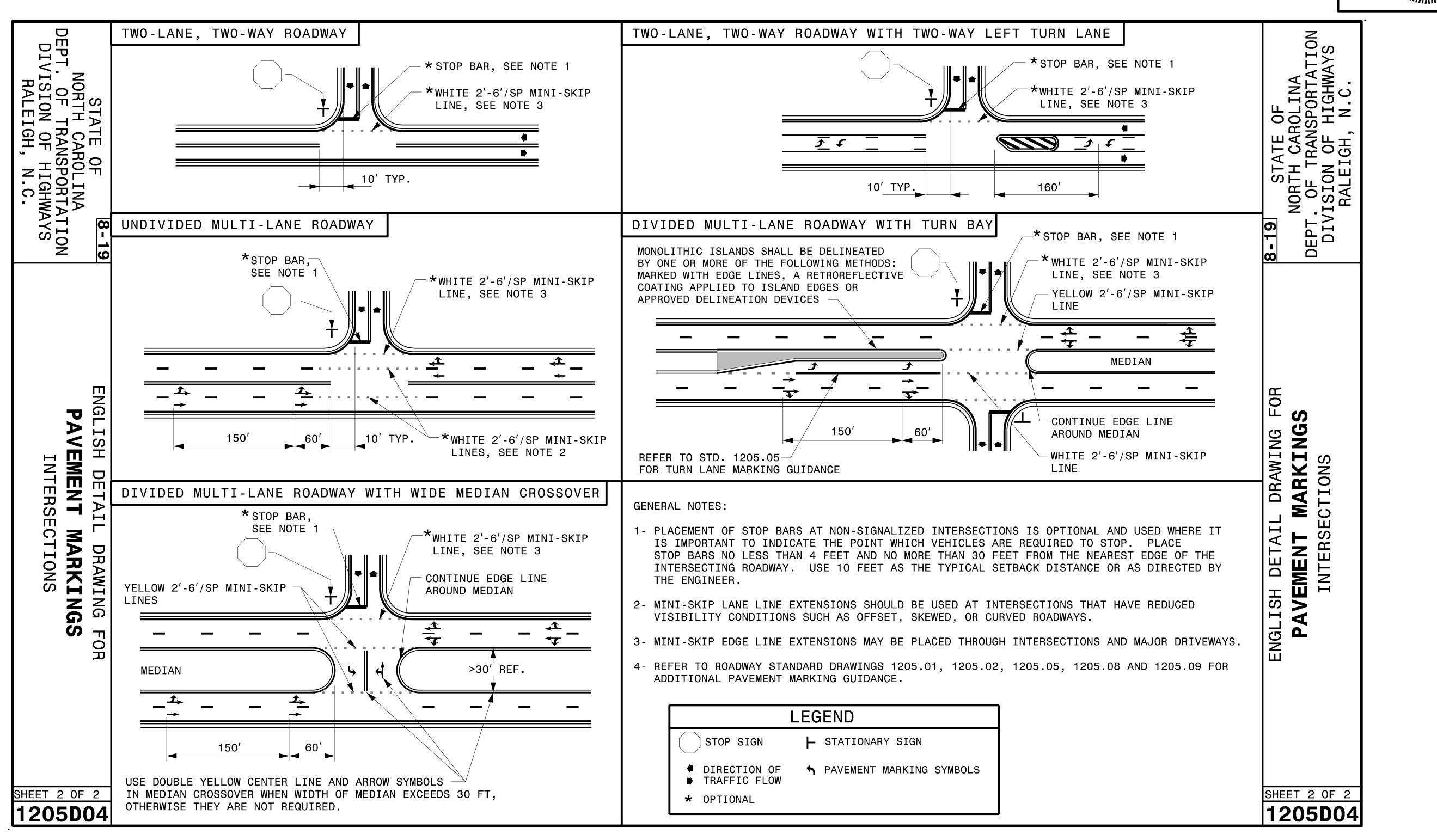
REVISED PAVEMENT MARKING ROADWAY STANDARD DRAWING
