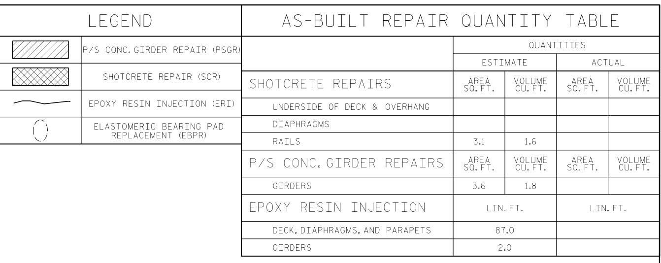
VALUES IN CHART REPRESENT ESTIMATED REPAIR TOTALS AFTER REMOVAL OF UNSOUND CONCRETE. MINIMUM OF 1"BEHIND REBAR AND MINIMUM 2"CLEARANCE TO SAWCUT. FOR REPAIR DETAILS, SEE "CONCRETE RESTORATION DETAILS" SHEETS.
