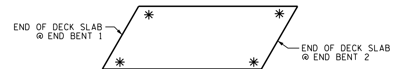
SKETCH SHOWING POINTS OF ATTACHMENT * LOCATION OF GUARDRAIL ATTACHMENT
