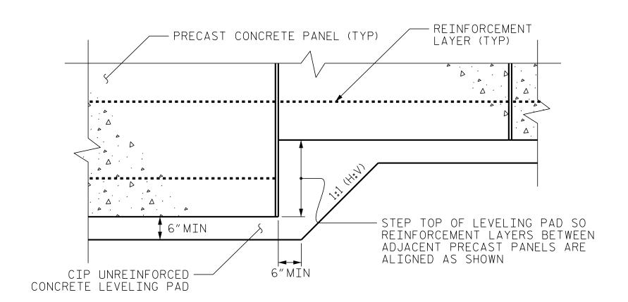
PRECAST PANELS LEVELING PAD STEP DETAIL
