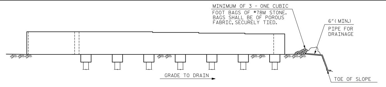
BAGGED STONE AND PIPE SHALL BE PLACED IMMEDIATELY AFTER COMPLETION OF END BENT EXCAVATION. PIPE MAY BE EITHER CONCRETE, CORRUGATED STEEL, CORRUGATED ALUMINUM ALLOY OR CORRUGATED PLASTIC. PERFORATED PIPE WILL NOT BE ALLOWED.
