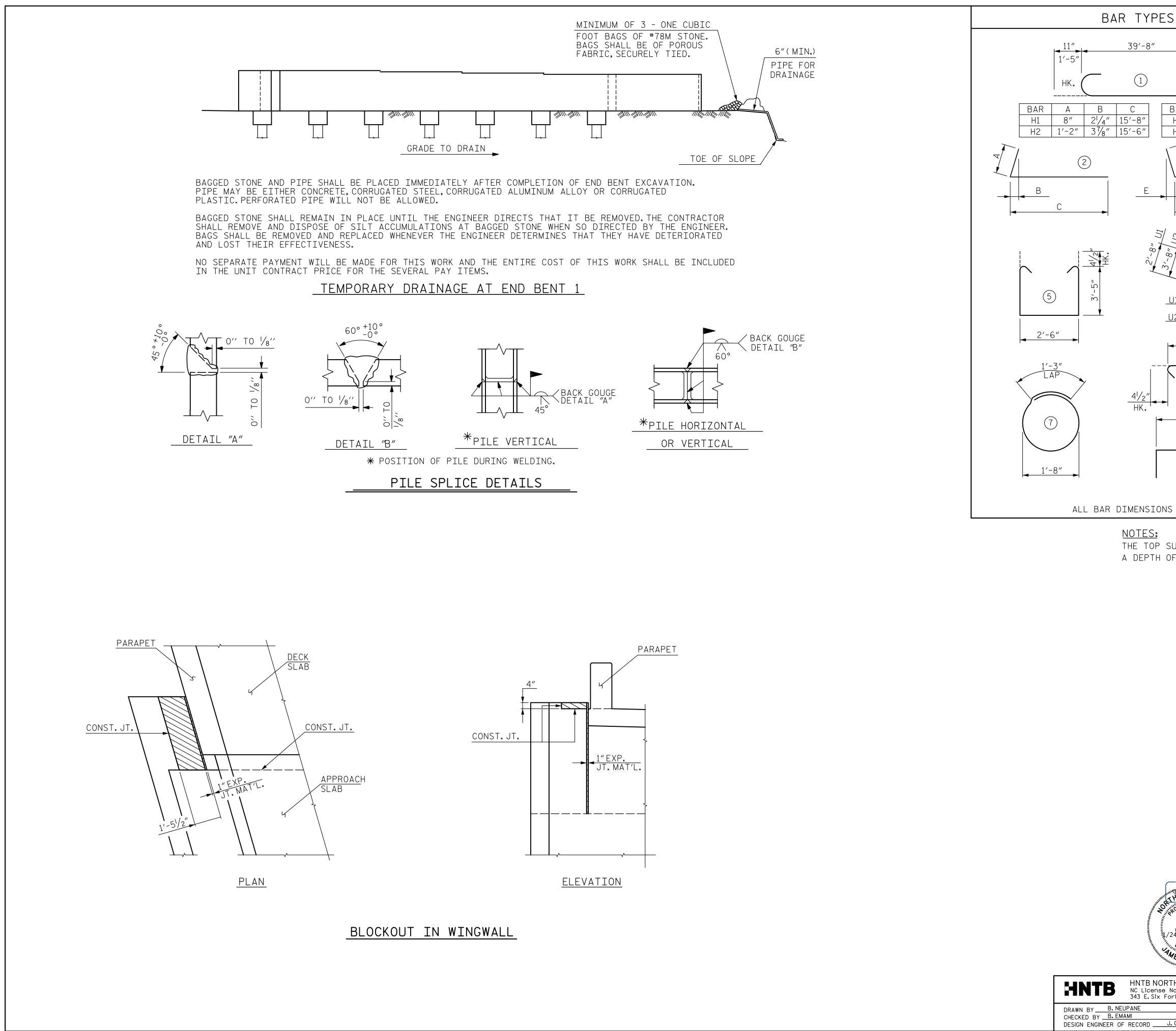
NOTES THE TOP SURFACE OF THE END BENT CAP, EXCEPT THE BEARING AREA, SHALL BE RAKED TO A DEPTH OF  $\frac{1}{4}$ ".
