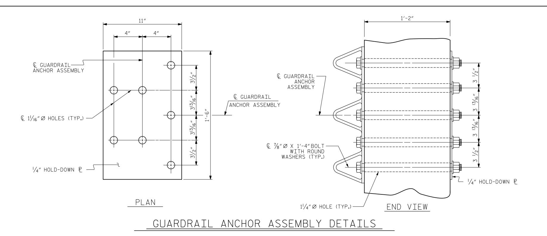
LOCATION OF GUARDRAIL ANCHOR AT END POST
