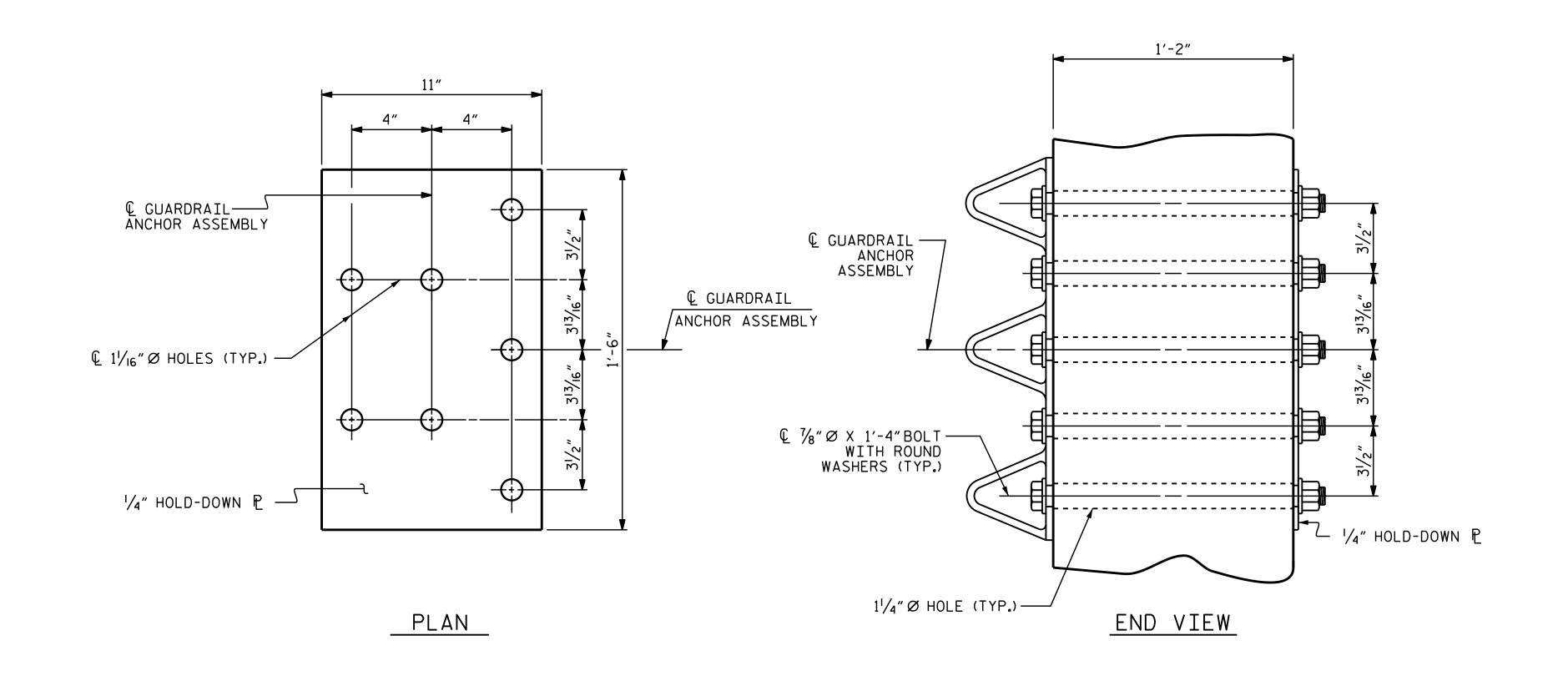
GUARDRAIL ANCHOR ASSEMBLY DETAILS
