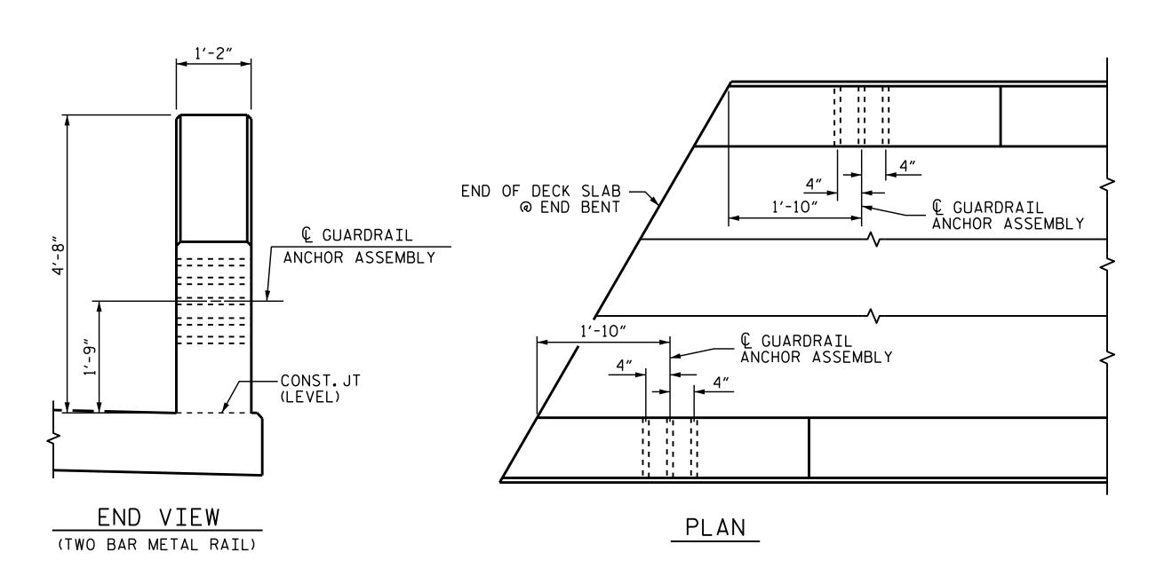
LOCATION OF GUARDRAIL ANCHOR AT END POST
