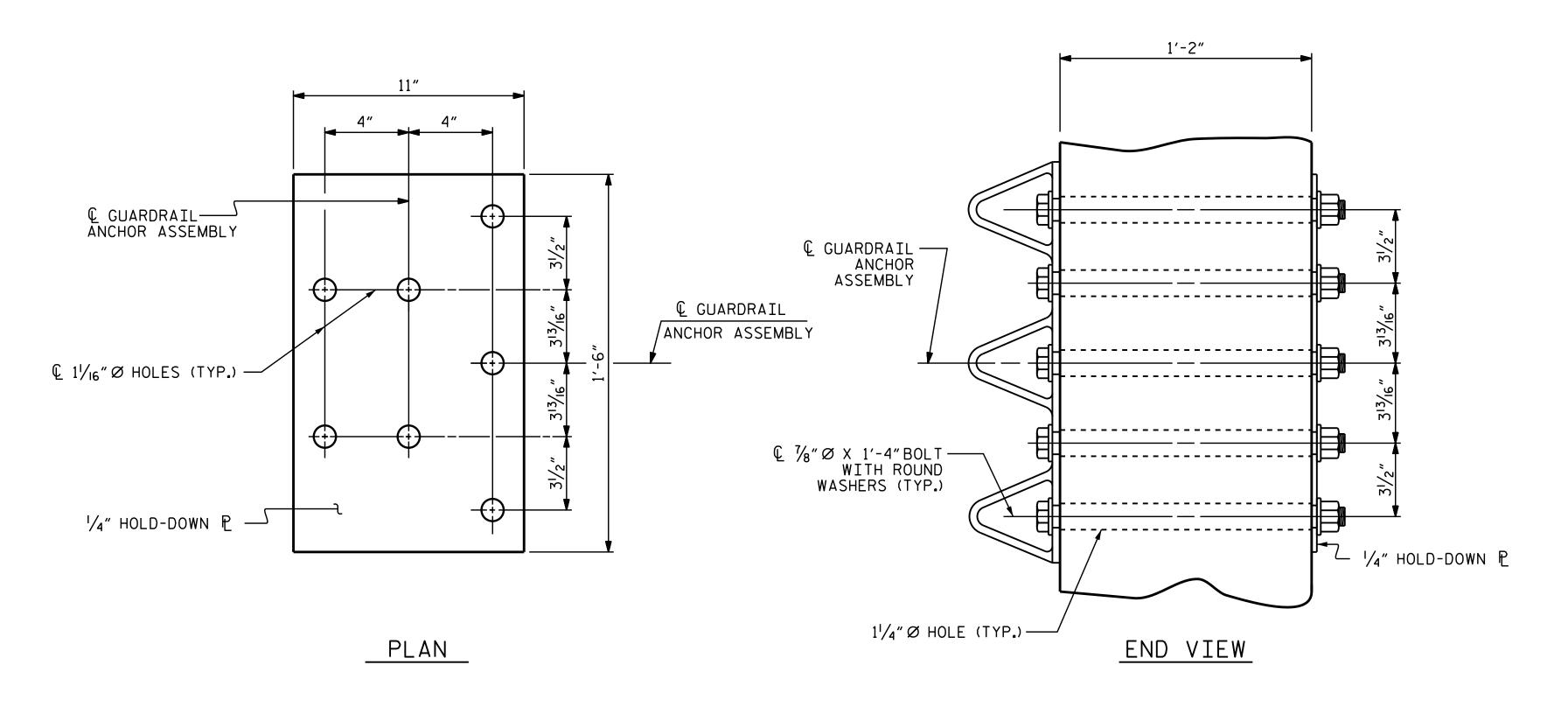
GUARDRAIL ANCHOR ASSEMBLY DETAILS
