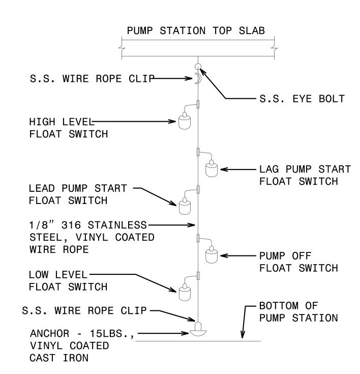
FLOAT SWITCH MOUNTING DETAIL
