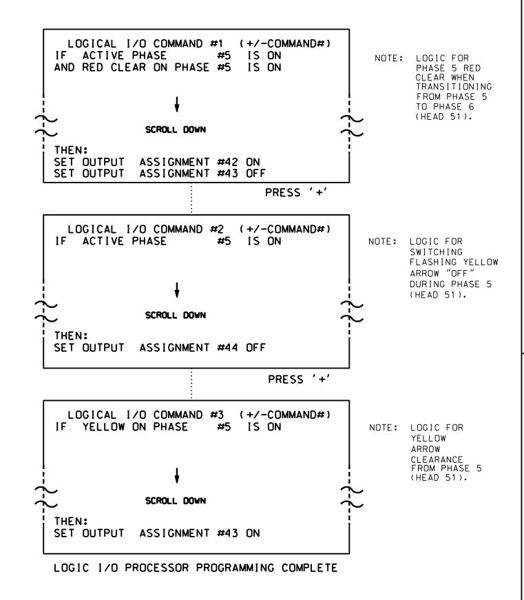
OUTPUT REFERENCE SCHEDULE USE TO INTERPRET LOGIC PROCESSOR OUTPUT 42 = Overlap C Red OUTPUT 43 = Overlap C Yellow OUTPUT 44 = Overlap C Green
