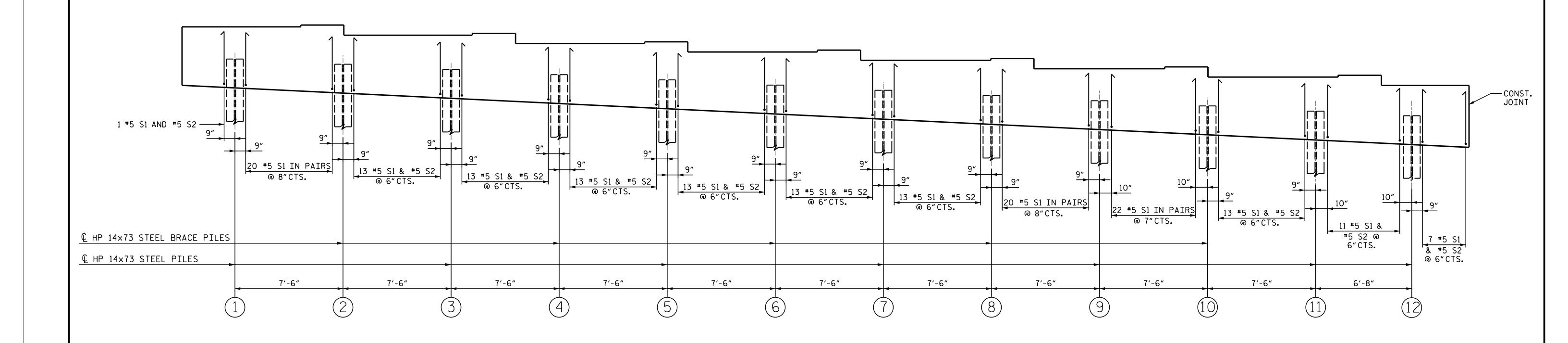
STIRRUP SPACING - END BENT 1 STAGE II
