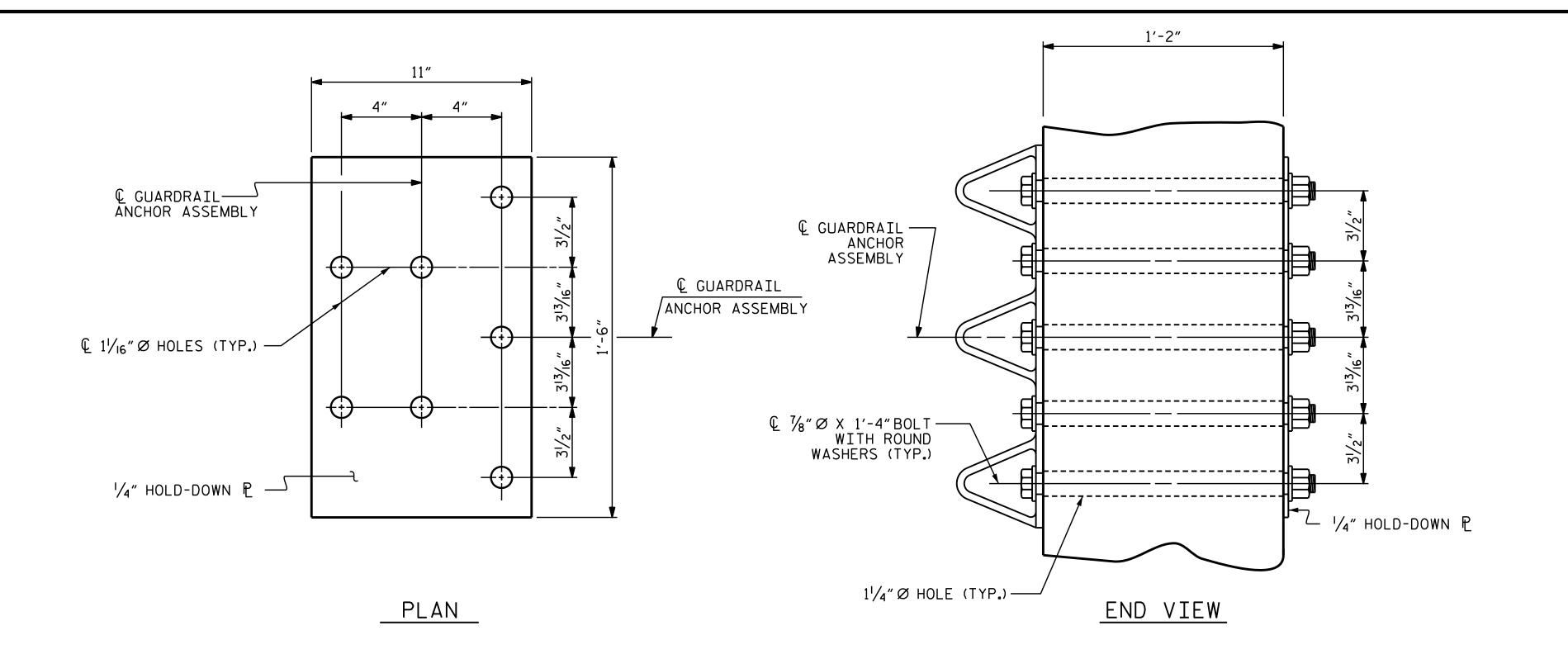
GUARDRAIL ANCHOR ASSEMBLY DETAILS
