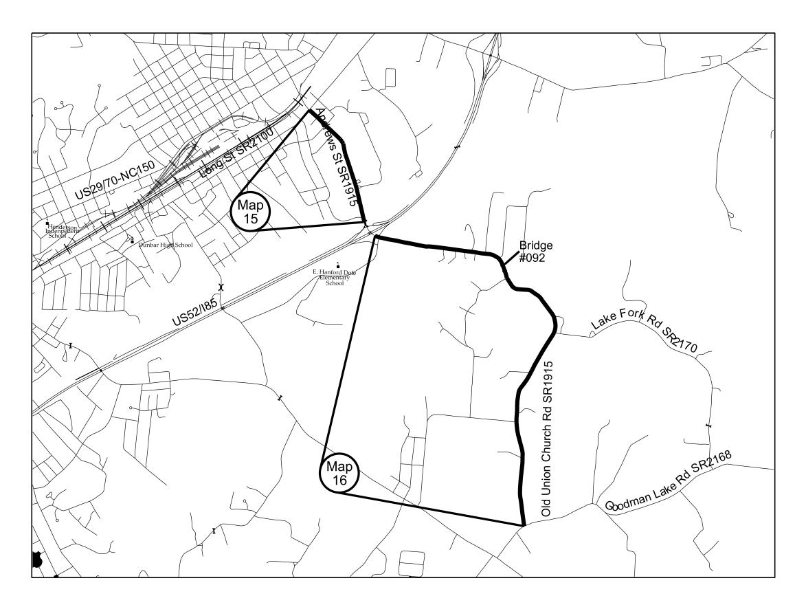
Map 15 Andrews St SR1915 from Long St SR2100 to concrete joint at US52/I85 Mill 11/2" depth entire width Mill 11/2" incidental milling at all SR Intersections Patching to be done by DOT forces Pave 11/2" S9.5B
