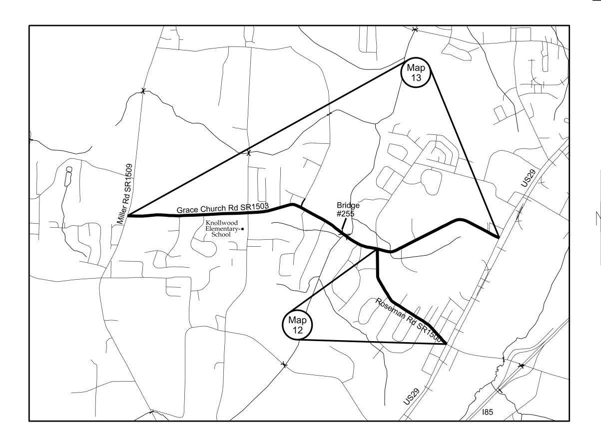
Map 12 Roseman Rd SR1500 from US29 to Grace Church Rd SR1503 Mill 0-11/2" incidental milling end, beginning and at all SR intersections Patching to be done by DOT forces Asphalt surface treament, Matcoat #78M stone Pave 11/2" S9.5B
