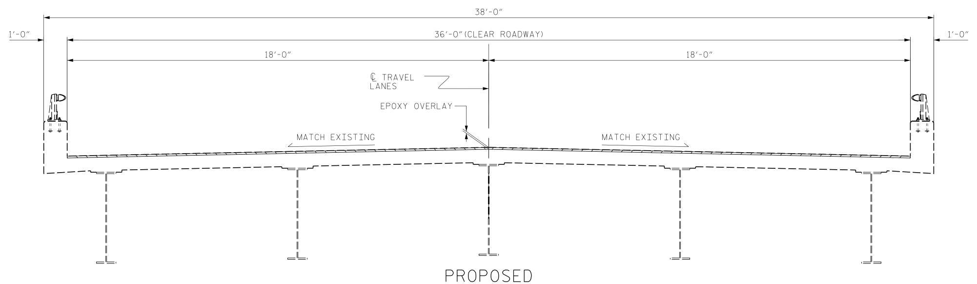
EXISTING EXISTING — DECK SURFACE 3/8" EPOXY OVERLAY FINISHED DECK SURFACE DECK SURFACE AFTER
