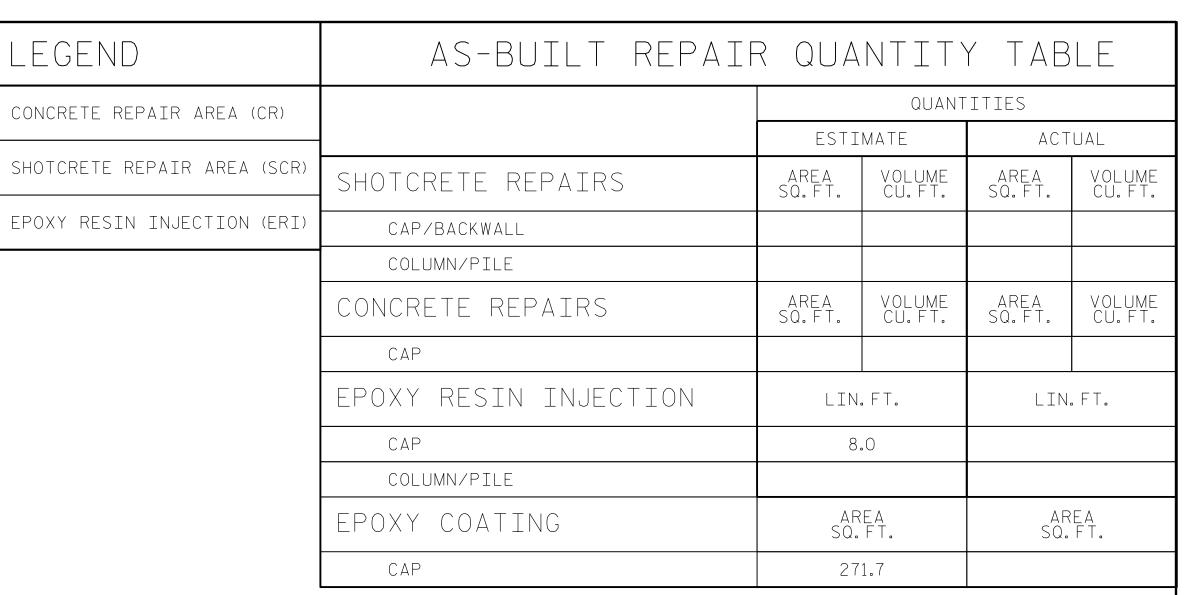
VALUES IN CHART REPRESENT ESTIMATED REPAIR TOTALS AFTER REMOVAL OF UNSOUND CONCRETE. MINIMUM OF 1"BEHIND REBAR AND MINIMUM 2"CLEARANCE TO SAWCUT. FOR REPAIR DETAILS, SEE "CONCRETE RESTORATION DETAILS" SHEETS.
