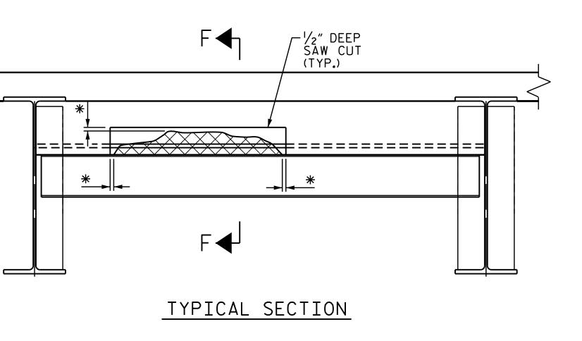
\* REMOVE CONCRETE UNTIL SOUND CONCRETE IS FOUND (2" MIN.CL.)
