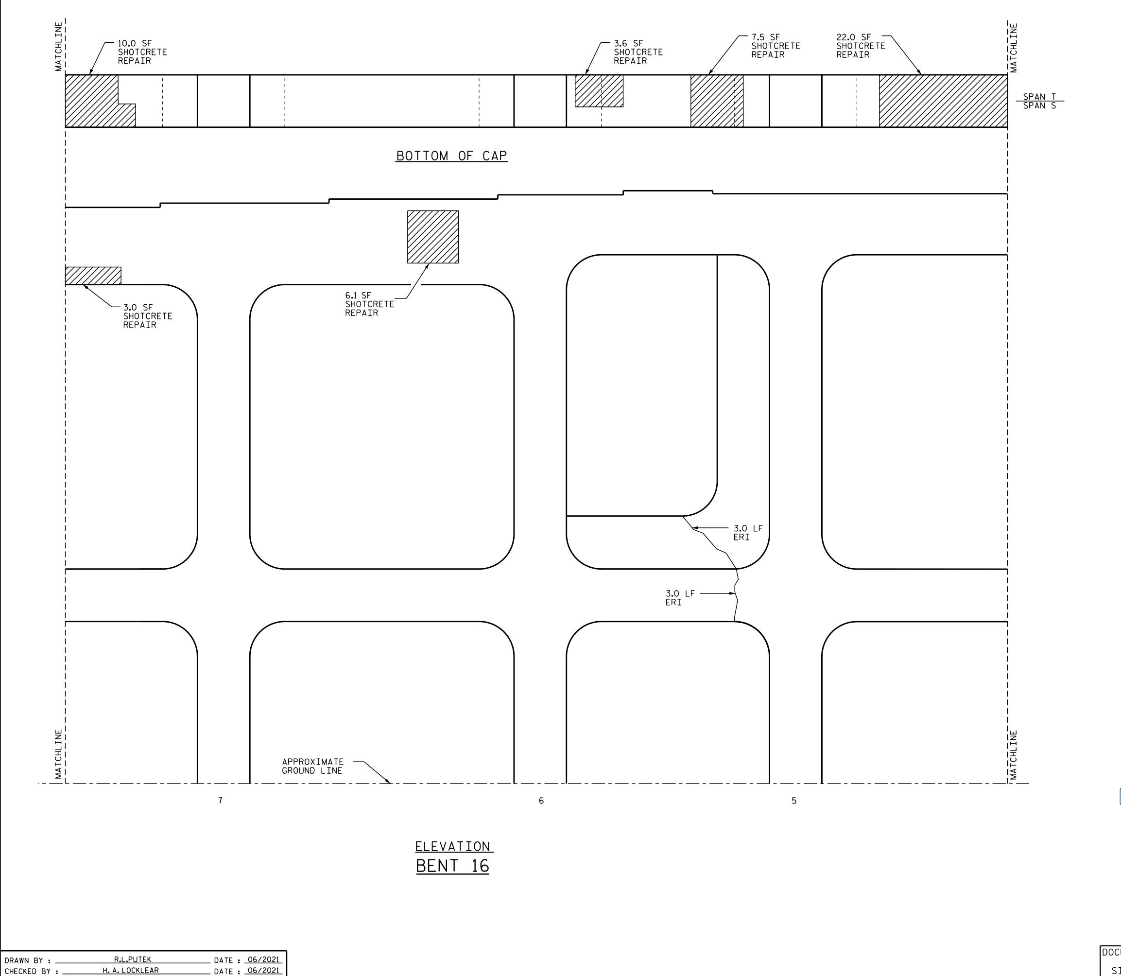
AS-BUILT REPAIR QUANTITY TABLE QUANTITIES BENT 16 ESTIMATE ACTUAL VOLUME AREA SQ.FT. VOLUME SHOTCRETE REPAIRS SQ.FT. CU.FT. CU.FT. 52.2 CAP 26.1 COLUMNS & STRUTS 0.0 0.0 VOLUME CONCRETE REPAIRS AREA VOLUME SQ.FT. CU.FT. SQ.FT. CU.FT. CAP 0.0 0.0 EPOXY RESIN INJECTION LIN.FT. LIN.FT. CAP 0.0 COLUMNS & STRUTS 6.0 EPOXY COATING SQ.FT. SQ.FT. TOP OF BENT CAP & STRUTS
