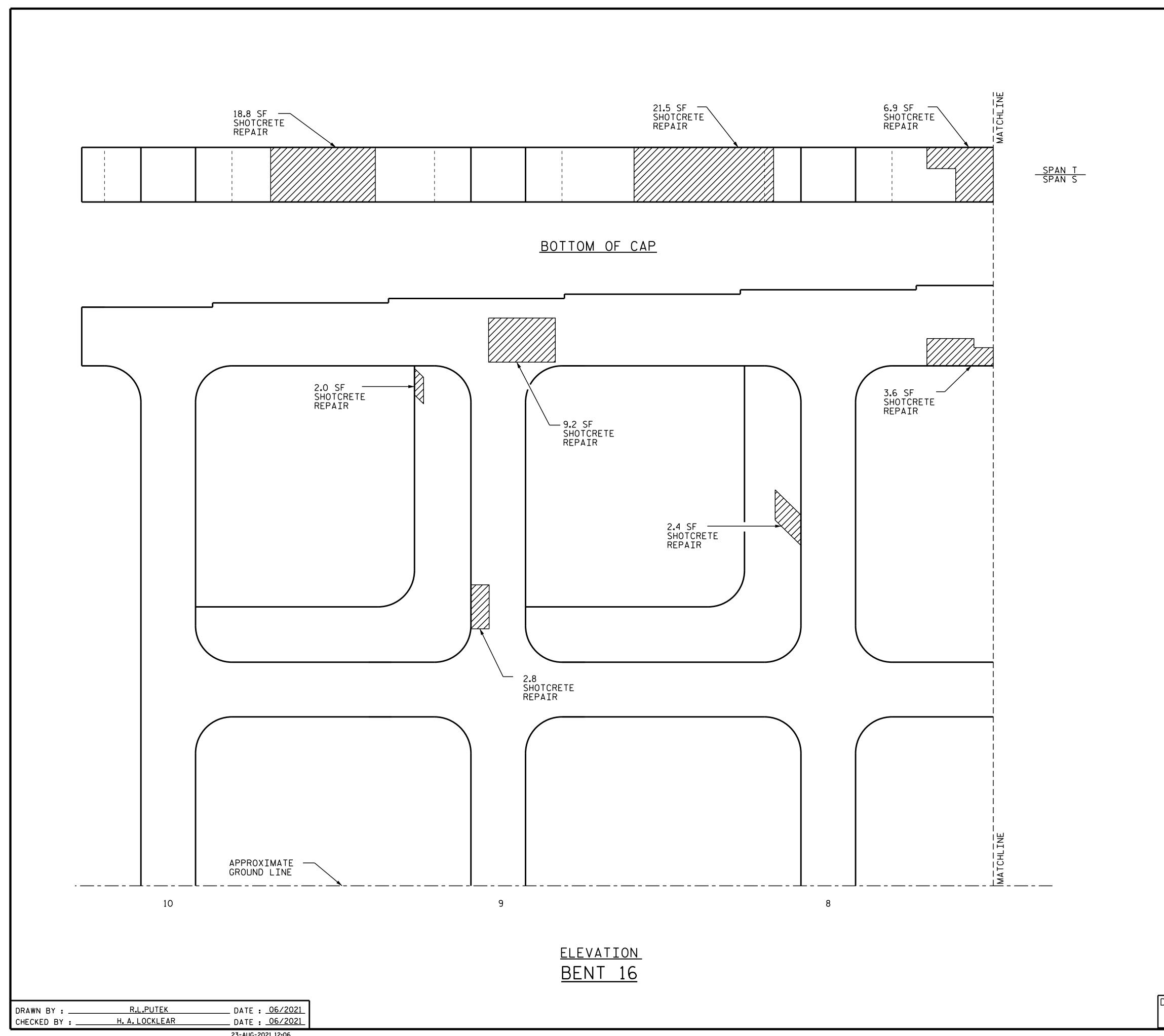
AS-BUILT REPAIR QUANTITY TABLE QUANTITIES BENT 16 ESTIMATE ACTUAL VOLUME AREA SQ.FT. VOLUME SHOTCRETE REPAIRS SO.FT. CU.FT. CU.FT. CAP 60.0 30.0 3.6 COLUMNS & STRUTS 7.2 VOLUME AREA VOLUME CONCRETE REPAIRS SQ.FT. CU.FT. SQ.FT. CU.FT. CAP 0.0 0.0 EPOXY RESIN INJECTION LIN.FT. LIN.FT. CAP 0.0 COLUMNS & STRUTS 0.0 EPOXY COATING SQ.FT. SQ.FT. TOP OF BENT CAP & STRUTS
