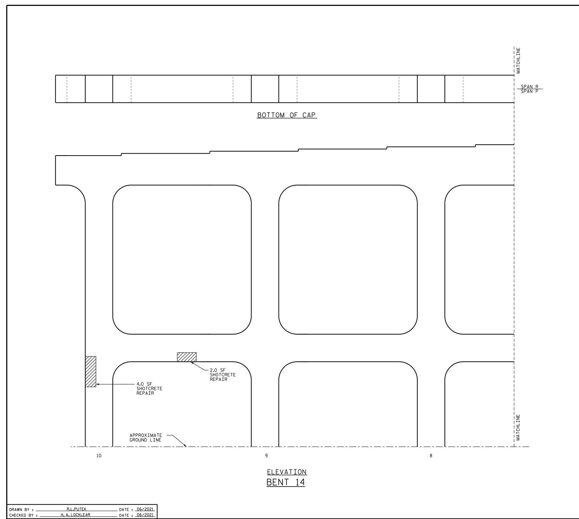
AS-BUILT REPAIR QUANTITY TABLE QUANTITIES BENT 14 ESTIMATE ACTUAL VOLUME AREA SQ.FT. VOLUME SHOTCRETE REPAIRS SQ.FT. CU.FT. CU.FT. 0.0 0.0 3.0 COLUMNS & STRUTS 6.0 VOLUME VOLUME CONCRETE REPAIRS SQ.FT. CU.FT. SQ.FT. CU.FT. 0.0 0.0 EPOXY RESIN INJECTION LIN.FT. LIN.FT. CAP 0.0 COLUMNS & STRUTS 0.0
