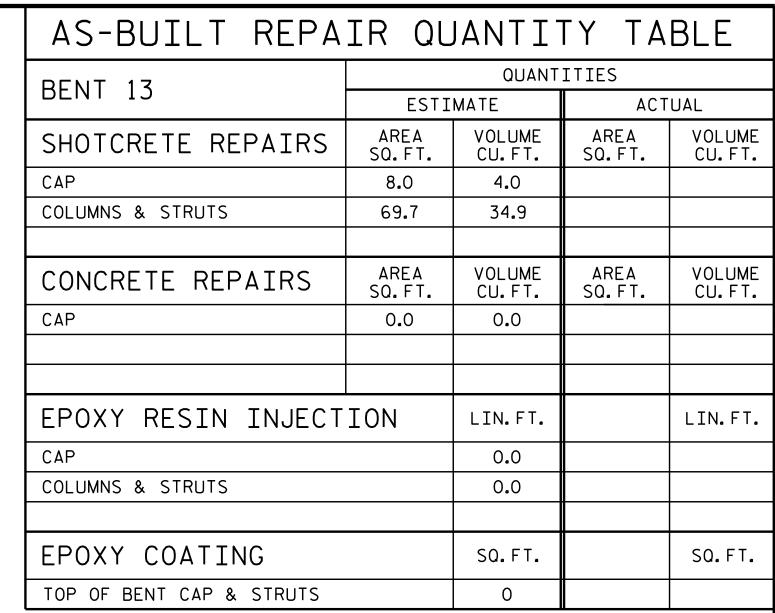
VALUES IN CHART REPRESENT ESTIMATED REPAIR TOTALS AFTER REMOVAL OF UNSOUND CONCRETE, MIN. OF 1" BEHIND REBAR AND 2" MIN. CLEAR TO SAWCUT. FOR REPAIR DETAILS, SEE "TYPICAL CAP AND COLUMN REPAIR DETAILS" SHEET.
