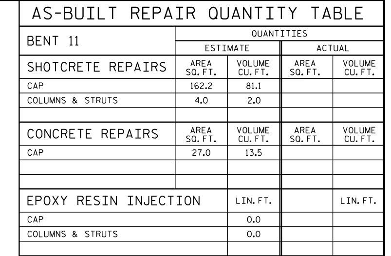
VALUES IN CHART REPRESENT ESTIMATED REPAIR TOTALS AFTER REMOVAL OF UNSOUND CONCRETE, MIN. OF 1" BEHIND REBAR AND 2" MIN. CLEAR TO SAWCUT. FOR REPAIR DETAILS, SEE "TYPICAL CAP AND COLUMN REPAIR DETAILS" SHEET.
