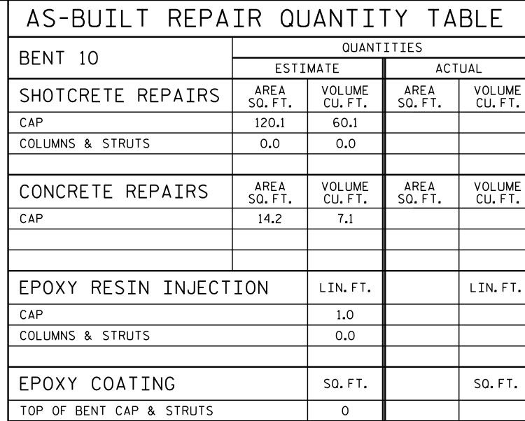
VALUES IN CHART REPRESENT ESTIMATED REPAIR TOTALS AFTER REMOVAL OF UNSOUND CONCRETE, MIN. OF 1" BEHIND REBAR AND 2" MIN. CLEAR TO SAWCUT. FOR REPAIR DETAILS, SEE "TYPICAL CAP AND COLUMN REPAIR DETAILS" SHEET.
