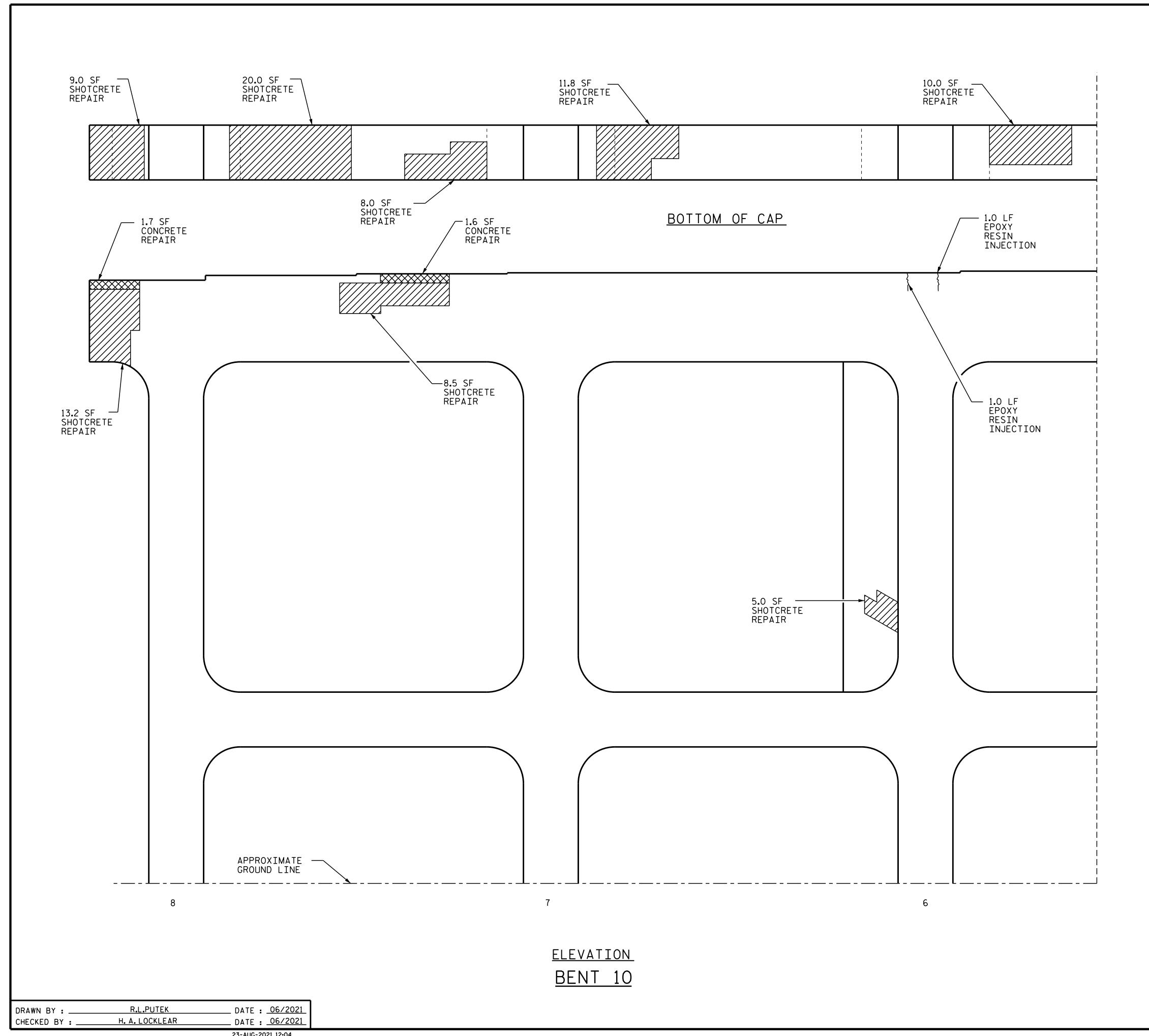
AS-BUILT REPAIR QUANTITY TABLE QUANTITIES BENT 10 ESTIMATE ACTUAL VOLUME AREA SQ.FT. VOLUME CU.FT. SHOTCRETE REPAIRS SQ.FT. CU.FT. 40.3 CAP 80.5 2.5 COLUMNS & STRUTS 5.0 AREA SQ.FT. VOLUME VOLUME CONCRETE REPAIRS CU.FT. SQ.FT. CU.FT. CAP 3.3 1.7 EPOXY RESIN INJECTION LIN.FT. LIN.FT. CAP 2.0 COLUMNS & STRUTS 0.0 EPOXY COATING SQ.FT. SQ.FT. TOP OF BENT CAP & STRUTS
