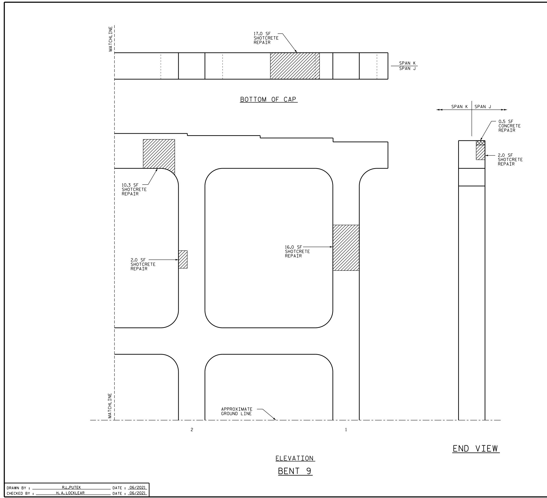
AS-BUILT REPAIR QUANTITY TABLE QUANTITIES BENT 9 ESTIMATE ACTUAL AREA SQ.FT. VOLUME CU.FT. VOLUME SHOTCRETE REPAIRS SQ.FT. CU.FT. 29.3 14.7 9.0 COLUMNS & STRUTS 18.0 AREA SQ.FT. VOLUME **VOLUME** CONCRETE REPAIRS CU.FT. SQ.FT. CU.FT. CAP 0.3 0.5 EPOXY RESIN INJECTION LIN.FT. LIN.FT. CAP 0.0 COLUMNS & STRUTS 0.0 EPOXY COATING SQ.FT. SQ.FT. TOP OF BENT CAP & STRUTS
