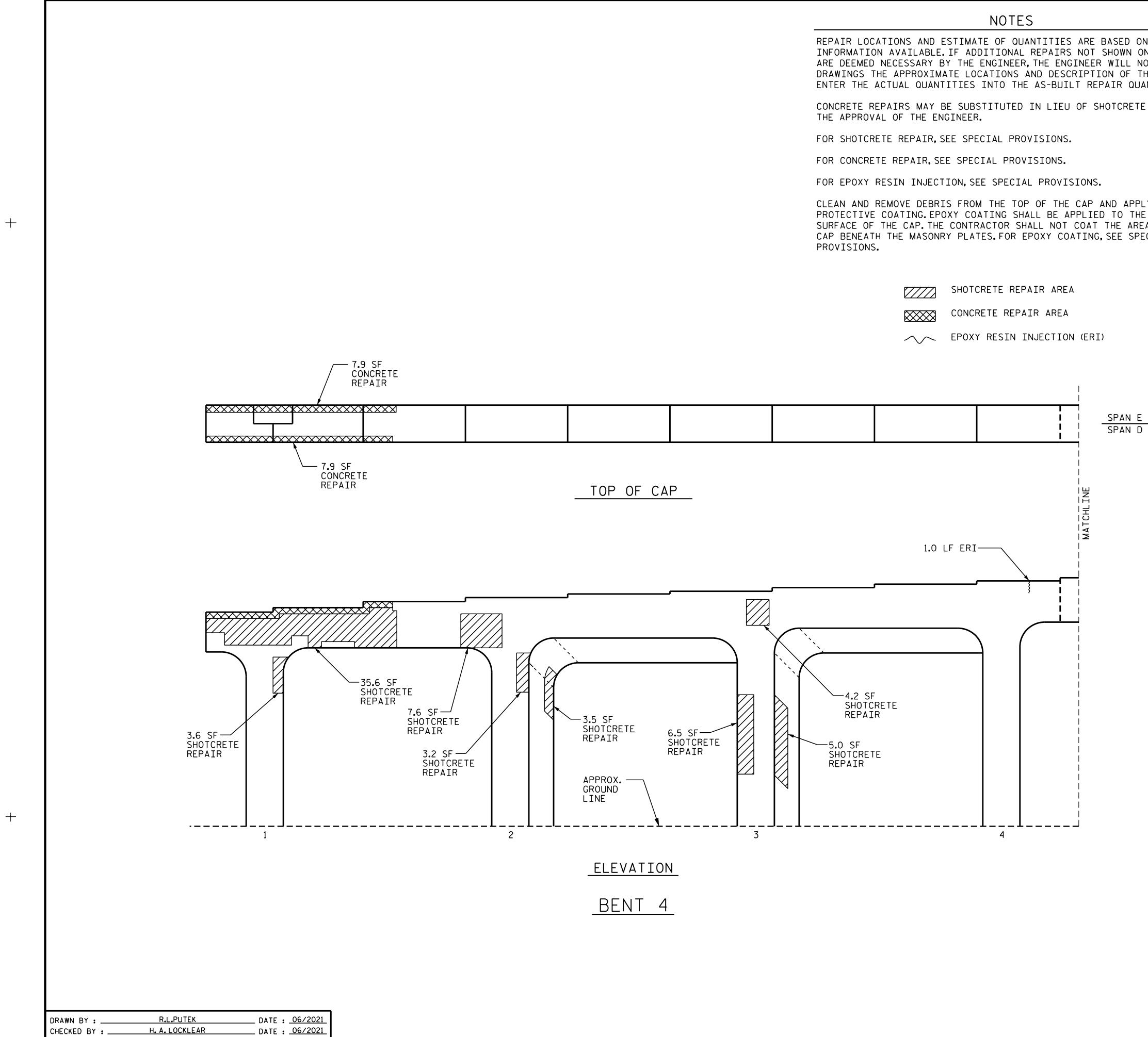
REPAIR LOCATIONS AND ESTIMATE OF QUANTITIES ARE BASED ON THE BEST INFORMATION AVAILABLE. IF ADDITIONAL REPAIRS NOT SHOWN ON THE DRAWING ARE DEEMED NECESSARY BY THE ENGINEER, THE ENGINEER WILL NOTE ON THE DRAWINGS THE APPROXIMATE LOCATIONS AND DESCRIPTION OF THE REPAIRS AND ENTER THE ACTUAL QUANTITIES INTO THE AS-BUILT REPAIR QUANTITY TABLE.
