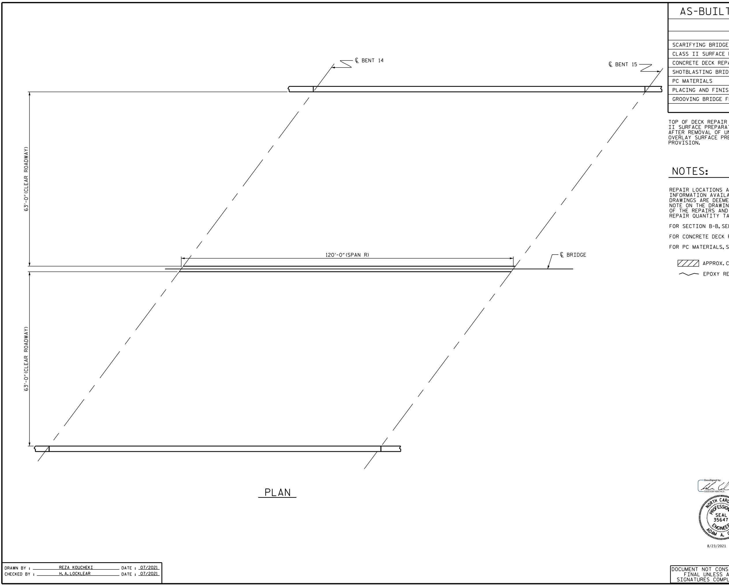
AS-BUILT REPAIR QUANTITY TABLE TOP OF DECK REPAIRS ESTIMATE ACTUAL 1680 SQ. YDS. SCARIFYING BRIDGE DECK 0.0 SQ. YDS. CLASS II SURFACE PREPARATION CONCRETE DECK REPAIR FOR PC OVERLAY 0.0 SQ. YDS. SHOTBLASTING BRIDGE DECK 1680 SQ. YDS. 151.6 CU. YDS. PLACING AND FINISHING PC OVERLAY 1680 SQ. YDS. 14400 SQ.FT. GROOVING BRIDGE FLOORS
