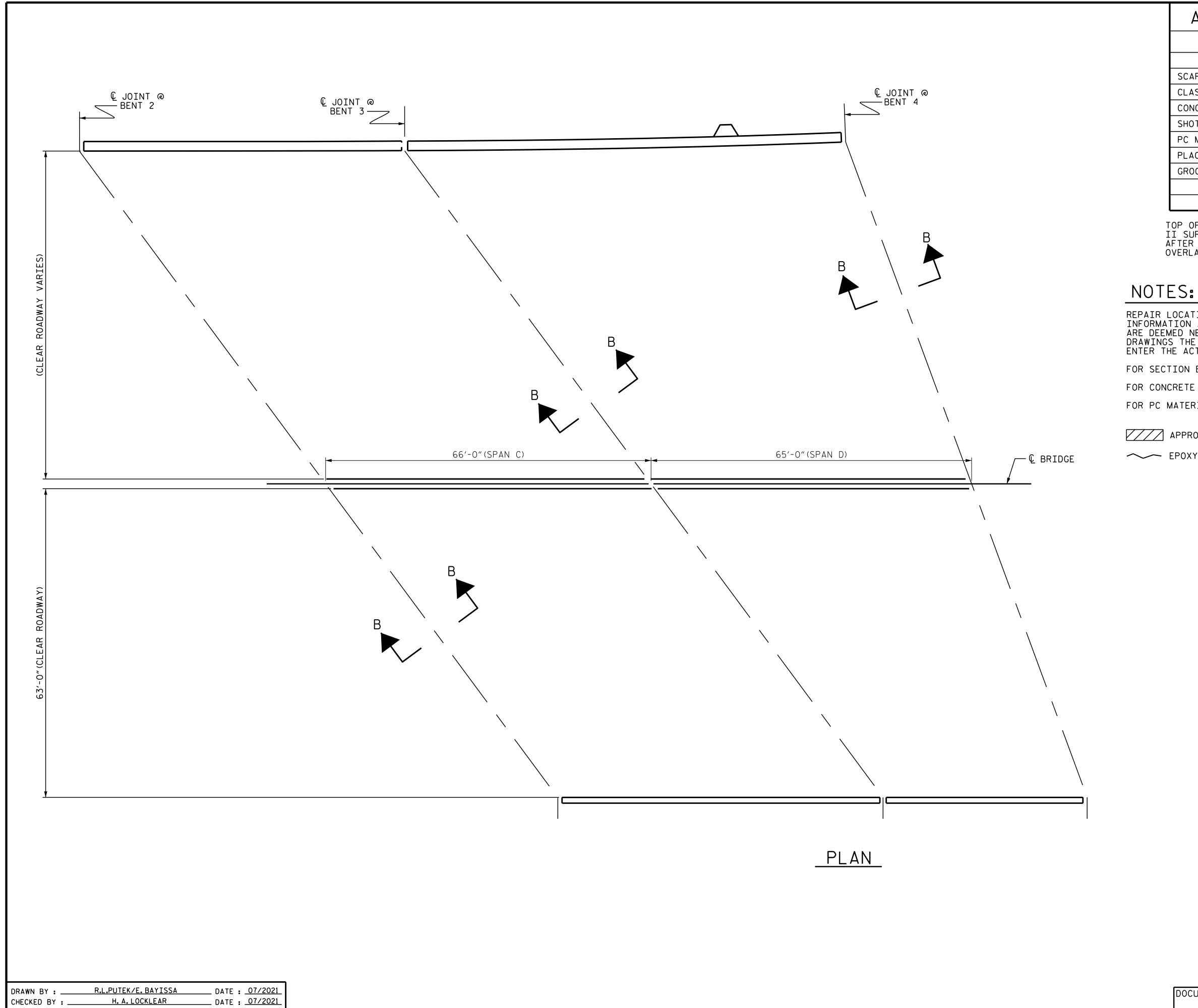
AS-BUILT REPAIR QUANTITY TABLE TOP OF DECK REPAIRS ESTIMATE ACTUAL SCARIFYING BRIDGE DECK 1915 SQ. YDS. 0.0 SQ. YDS. CLASS II SURFACE PREPARATION CONCRETE DECK REPAIR FOR PC OVERLAY 0.0 SQ. YDS. 1915 SQ. YDS. SHOTBLASTING BRIDGE DECK PC MATERIALS 93.1 CU. YDS. 1915 SQ. YDS. PLACING AND FINISHING PC OVERLAY 16296 SQ.FT. GROOVING BRIDGE FLOORS
