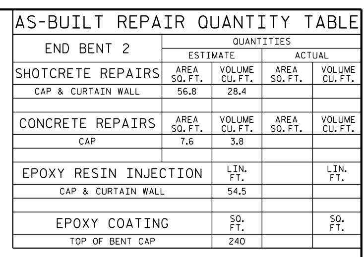
VALUES IN CHART REPRESENT ESTIMATED REPAIR TOTALS AFTER REMOVAL OF UNSOUND CONCRETE, MINIMUM OF 1"BEHIND REBAR AND MINIMUM 2"CLEARANCE TO SAWCUT. FOR REPAIR DETAILS, SEE "TYPICAL CAP AND COLUMN REPAIR DETAILS" SHEET.
