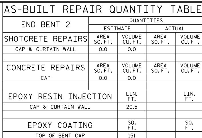
VALUES IN CHART REPRESENT ESTIMATED REPAIR TOTALS AFTER REMOVAL OF UNSOUND CONCRETE, MINIMUM OF 1"BEHIND REBAR AND MINIMUM 2"CLEARANCE TO SAWCUT. FOR REPAIR DETAILS, SEE "TYPICAL CAP AND COLUMN REPAIR DETAILS" SHEET.
