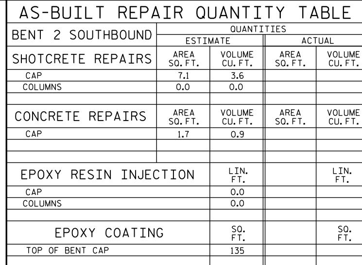
VALUES IN CHART REPRESENT ESTIMATED REPAIR TOTALS AFTER REMOVAL OF UNSOUND CONCRETE, MINIMUM OF 1"BEHIND REBAR AND MINIMUM 2"CLEARANCE TO SAWCUT. FOR REPAIR DETAILS, SEE "TYPICAL CAP AND COLUMN REPAIR DETAILS" SHEET.
