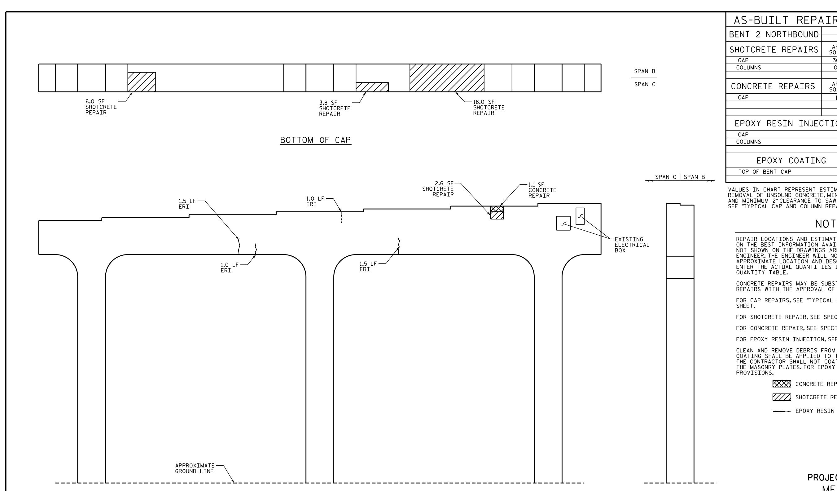
AS-BUILT REPAIR QUANTITY TABLE QUANTITIES ESTIMATE ACTUAL AREA VOLUME VOLUME CU.FT. SQ.FT. SQ.FT. CU.FT. 30.4 15.2 0.0 0.0 VOLUME SQ.FT. CU.FT. SQ.FT. CU.FT. 0.6 1.1 LIN. LIN. EPOXY RESIN INJECTION FT. FT. 5.0 0.0 SQ. FT. SQ. FT. 0
