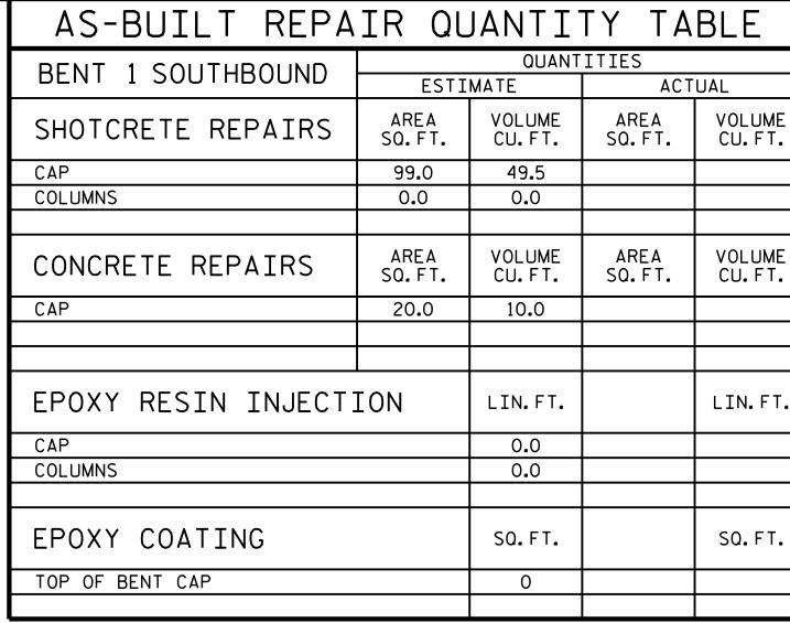
VALUES IN CHART REPRESENT ESTIMATED REPAIR TOTALS AFTER REMOVAL OF UNSOUND CONCRETE, MINIMUM OF 1"BEHIND REBAR AND MINIMUM 2"CLEARANCE TO SAWCUT. FOR REPAIR DETAISL, SEE "TYPICAL CAP AND COLUMNREPAIR DETAILS" SHEET.
