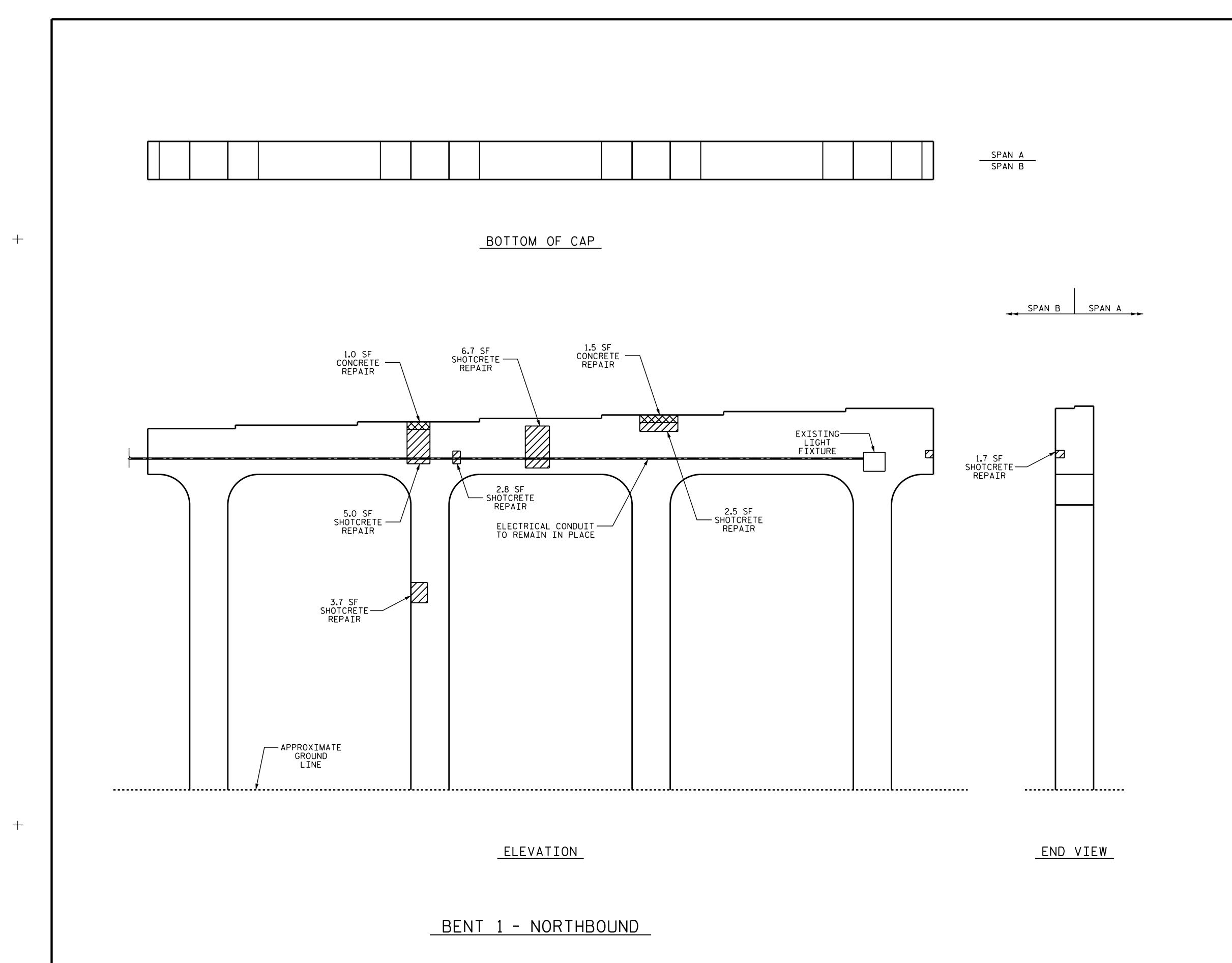
AS-BUILT REPAIR QUANTITY TABLE QUANTITIES BENT 1 NORTHBOUND ESTIMATE ACTUAL VOLUME CU.FT. **VOLUME** SHOTCRETE REPAIRS SO.FT. SQ.FT. CU.FT. CAP 18.7 9.4 COLUMNS 3.7 1.9 VOLUME CU.FT. **VOLUME** CONCRETE REPAIRS CU. FT. SQ.FT. SQ.FT. CAP 2.5 1.3 EPOXY RESIN INJECTION LIN.FT. LIN.FT. CAP 0.0 0.0 COLUMNS EPOXY COATING SQ.FT. SQ.FT. TOP OF BENT CAP 0
