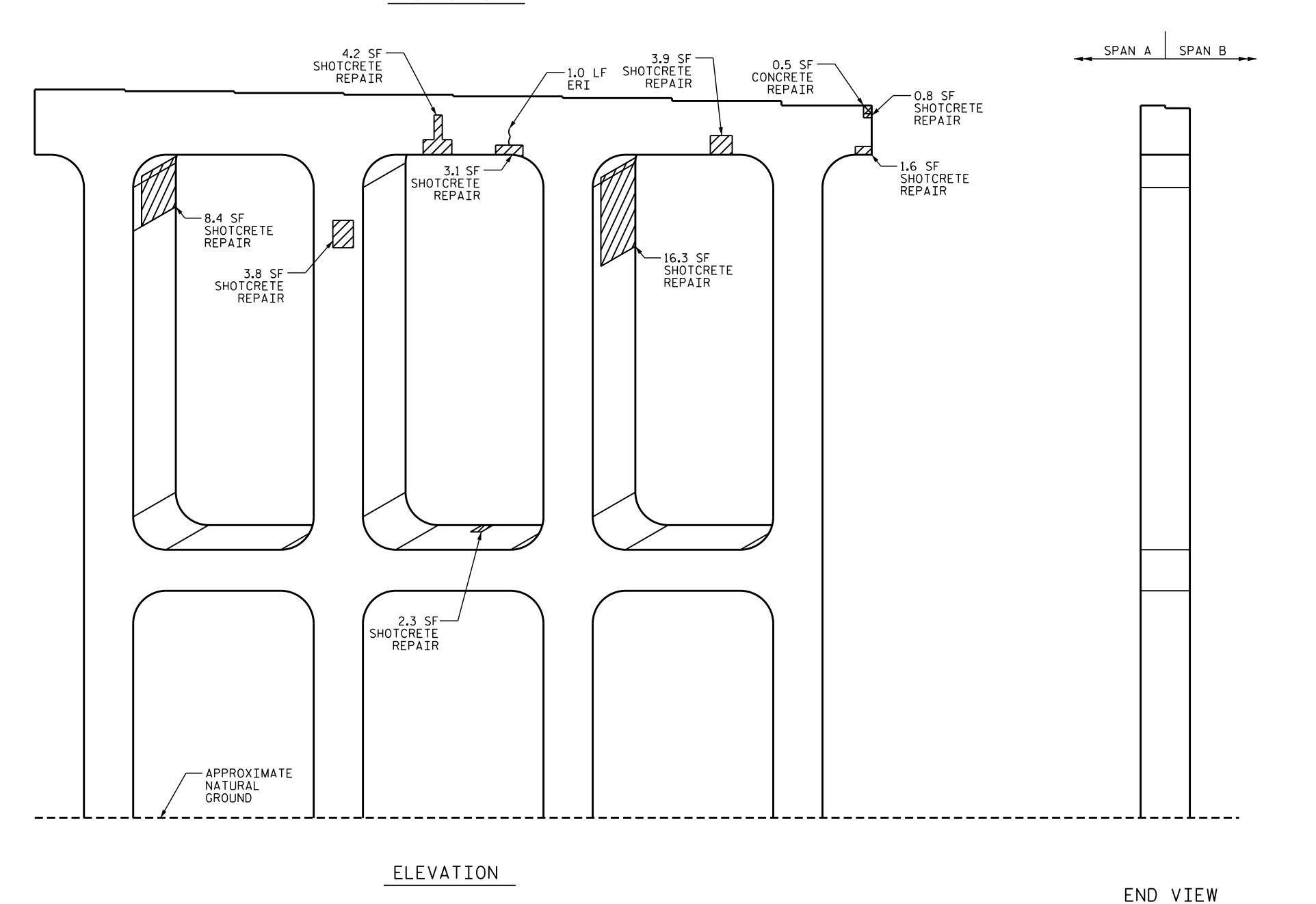
AS-BUILT REPAIR QUANTITY TABLE QUANTITIES BENT 1 SOUTHBOUND ESTIMATE ACTUAL AREA VOLUME VOLUME SHOTCRETE REPAIRS CU. FT. SQ.FT. SQ.FT. CU.FT. CAP 13.6 6.8 COLUMN & STRUTS 30.8 15.4 VOLUME VOLUME CONCRETE REPAIRS SQ.FT. CU.FT. SQ.FT. CU.FT. CAP 13.1 6.6 COLUMN & STRUTS 0.0 0.0 LIN. LIN. EPOXY RESIN INJECTION FT. 1.0 CAP COLUMN & STRUTS 0.0 SQ. FT. SQ. EPOXY COATING FT. TOP OF BENT CAP & STRUTS 276
