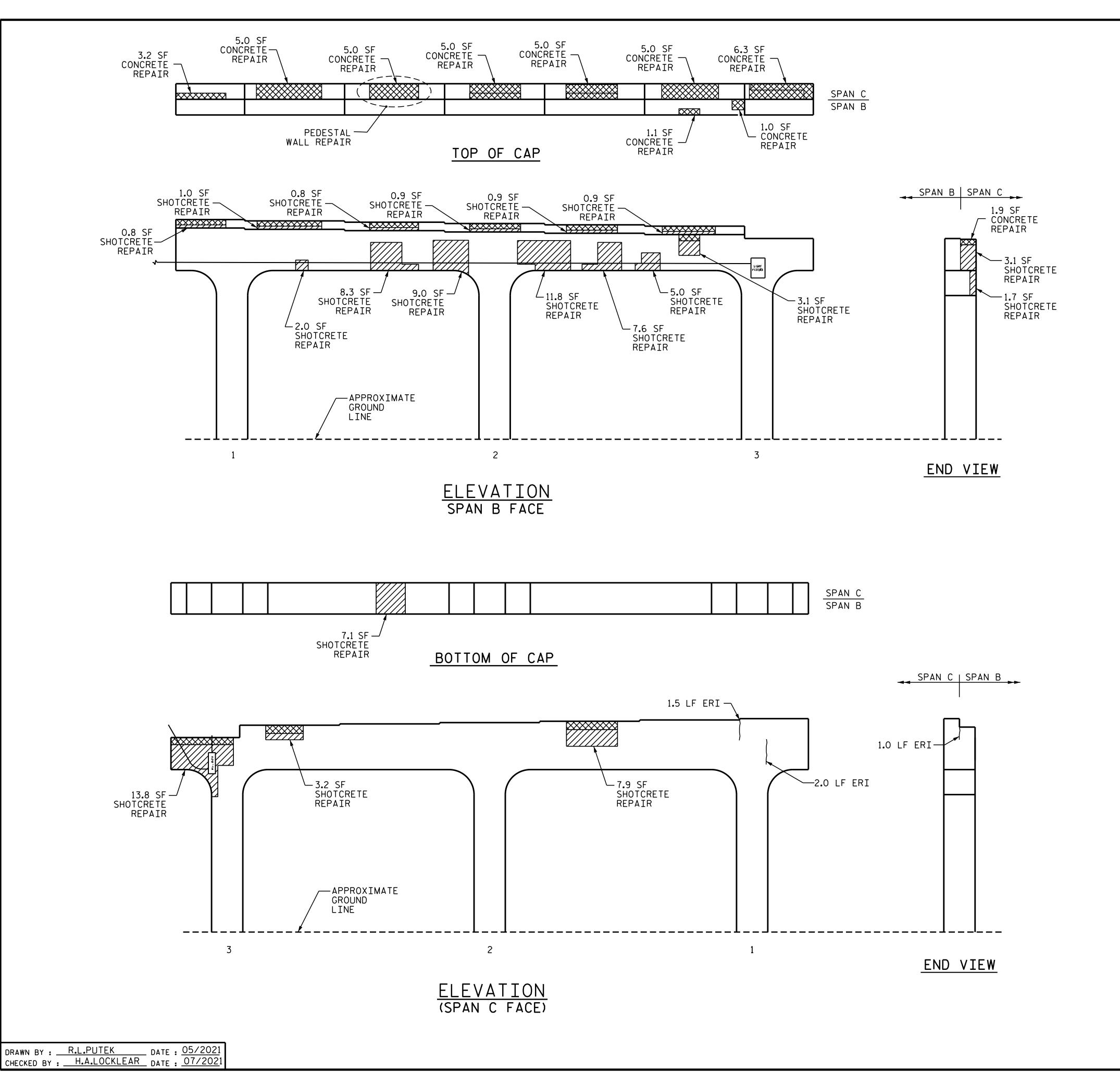
AS-BUILT REPAIR QUANTITY TABLE QUANTITIES |BENT 2 (SOUTHBOUND)| ESTIMATE ACTUAL VOLUME CU.FT. VOLUME SHOTCRETE REPAIRS SQ.FT. SQ.FT. CU.FT. CAP 89.1 44.6 COLUMNS 1.7 0.9 VOLUME **VOLUME** CONCRETE REPAIRS SQ.FT. SQ.FT. CU.FT. CU.FT. 30.7 CAP 46.0 EPOXY RESIN INJECTION LIN.FT. LIN.FT CAP 4.5 COLUMNS 0.0 EPOXY COATING SQ.FT. SQ.FT. TOP OF BENT CAP
