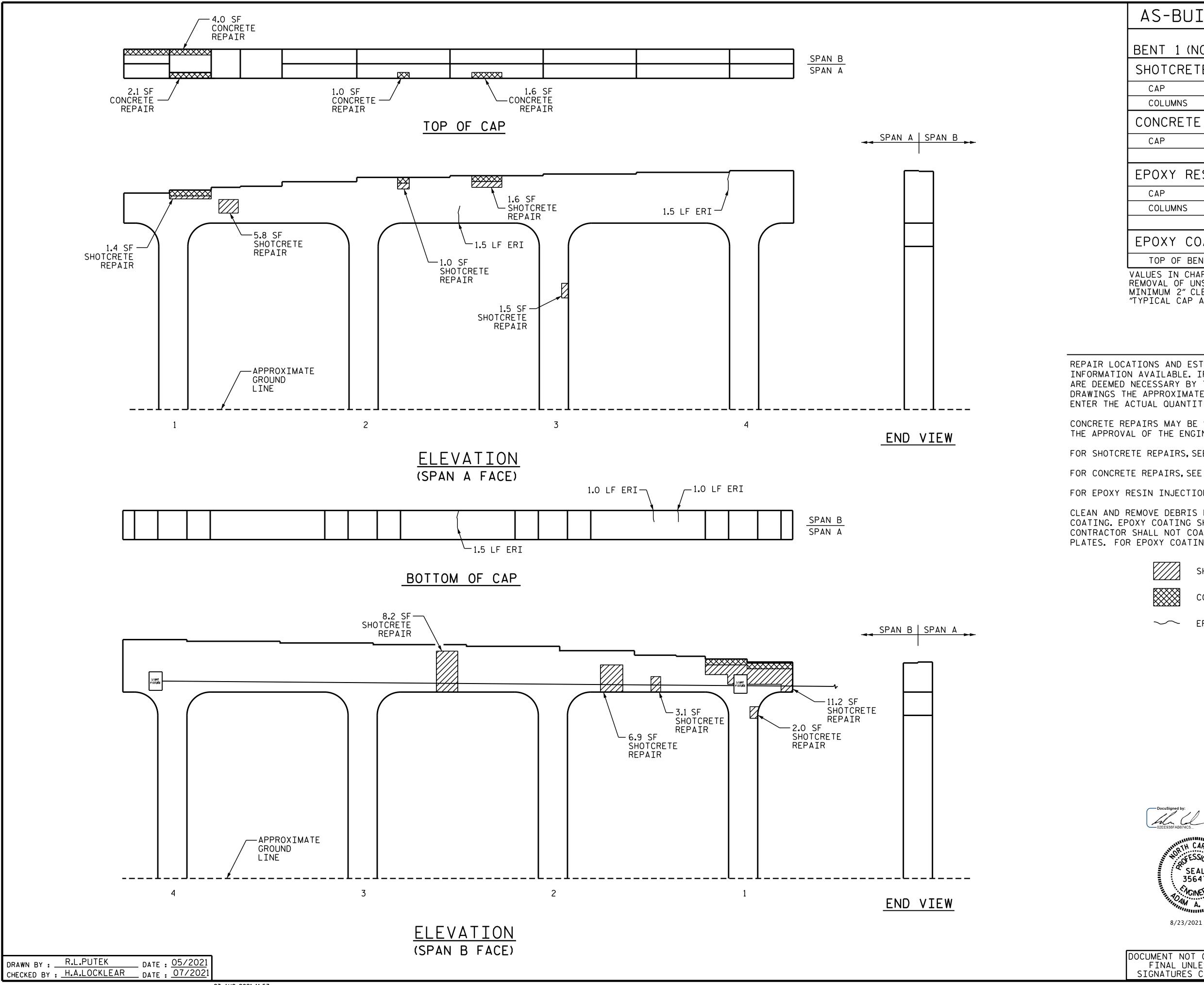
AS-BUILT REPAIR QUANTITY TABLE QUANTITIES BENT 1 (NORTHBOUND) ESTIMATE ACTUAL VOLUME CU.FT. VOLUME SHOTCRETE REPAIRS SQ.FT. SQ.FT. CU.FT. 39.2 19.6 3**.**5 COLUMNS 1.8 AREA **VOLUME VOLUME** CONCRETE REPAIRS SQ.FT. SQ.FT. CU.FT. CU.FT. 8.7 4.4 EPOXY RESIN INJECTION LIN.FT. LIN.FT 6.4 COLUMNS 0.0 EPOXY COATING SQ.FT. SQ.FT. TOP OF BENT CAP
