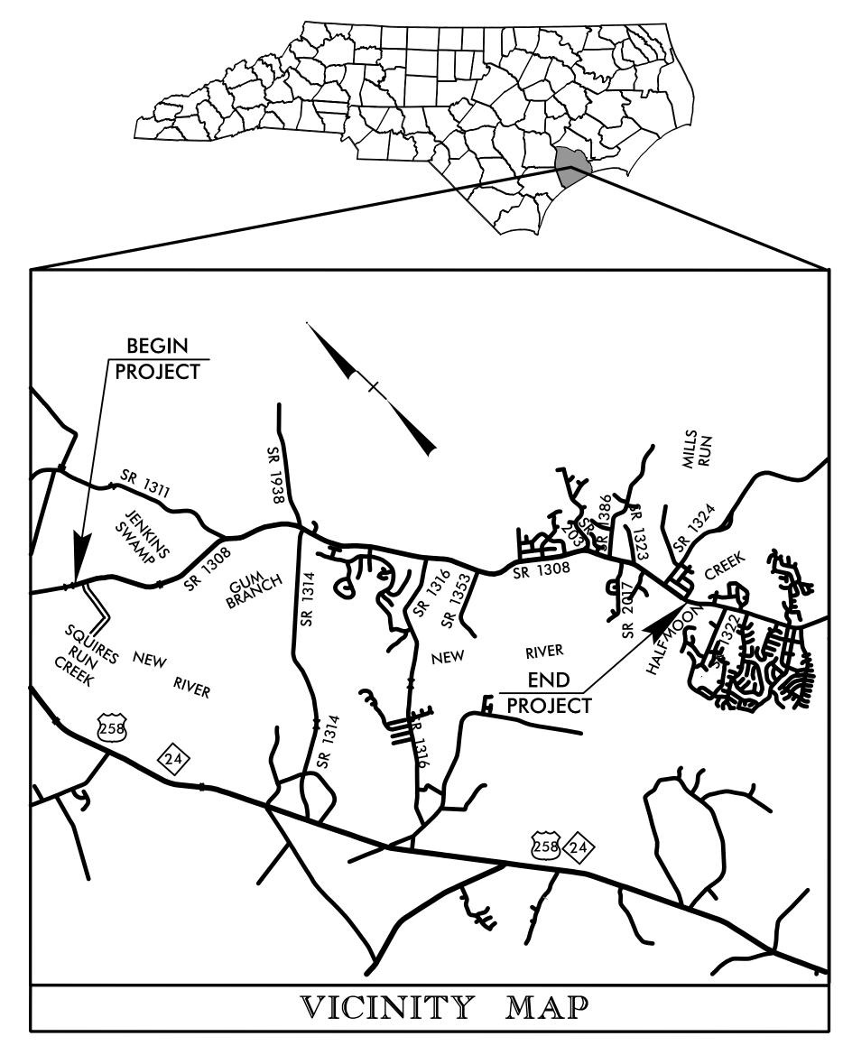
LOCATION: GUM BRANCH ROAD (SR 1308) - WIDENING FROM THE WEST OF MILLS FIELDS RD (SR 1313) TO EAST OF RAMSEY ROAD (SR 1324) TYPE OF WORK: GRADING, PAVING, DRAINAGE, AND SIGNALS
