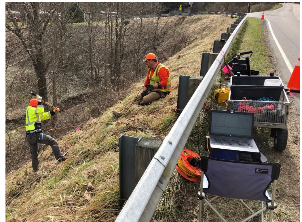
D. Photograph of seismic refraction data collection with sledgehammer source.
