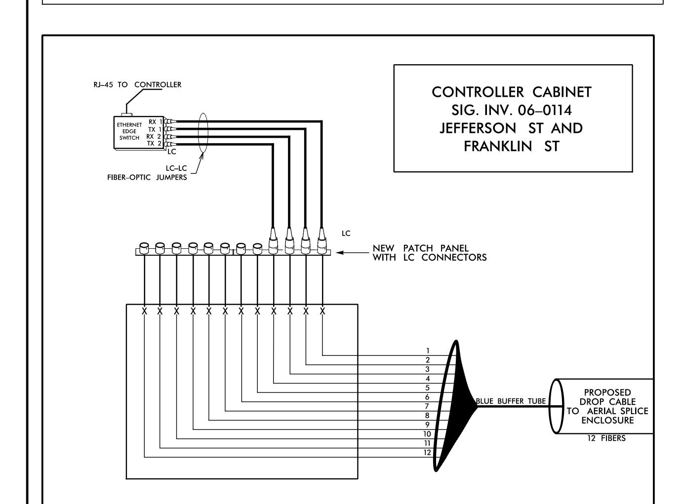
LEGEND COLOR CODE TIA/EIA 598-A X = FUSION SPLICE INDIVIDUAL FIBER (7) RED (1) BLUE C = CAP AND SEAL(2) ORANGE (8) BLACK EXPRESS ENTIRE BUFFER TUBE /FIBERS (3) GREEN (9) YELLOW **EXPRESS** THROUGH WITHOUT CUTTING (4) BROWN (10) VIOLET BUFFER SPLICE = SPLICE ALL FIBERS IN BUFFER (11) ROSE (5) SLATE TUBE COLOR TO COLOR (12) AQUA (6) WHITE
