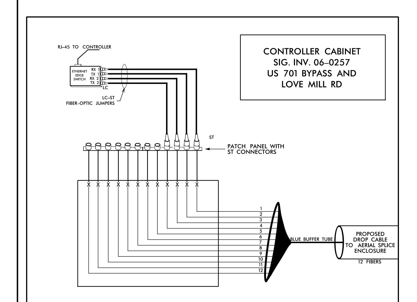
LEGEND COLOR CODE X = FUSION SPLICE INDIVIDUAL FIBER TIA/EIA 598-A (7) RED (1) BLUE C = CAP AND SEAL(2) ORANGE (8) BLACK EXPRESS ENTIRE BUFFER TUBE /FIBERS (3) GREEN (9) YELLOW **EXPRESS** THROUGH WITHOUT CUTTING (4) BROWN (10) VIOLET (11) ROSE SPLICE ALL FIBERS IN BUFFER (5) SLATE BUFFER SPLICE = TUBE COLOR TO COLOR (6) WHITE (12) AQUA
