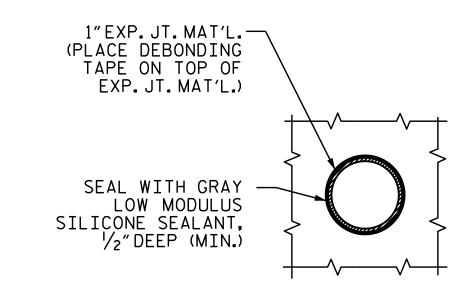
PLAN WHERE CONCRETE SLOPE PROTECTION MUST BE PLACED AROUND A BENT PILE
