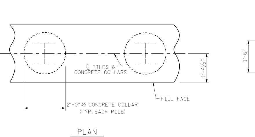
CORROSION PROTECTION FOR STEEL PILES DETAIL
